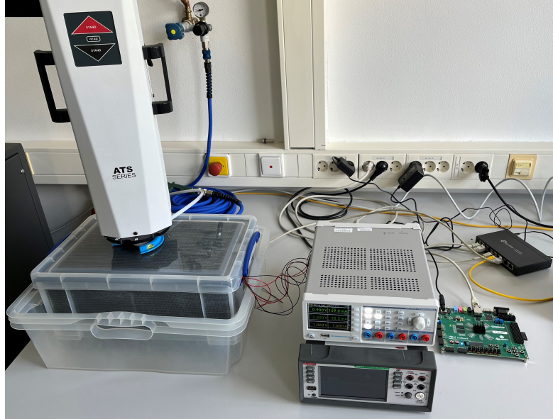
Figure 6.1: Setup of the leakage current test
