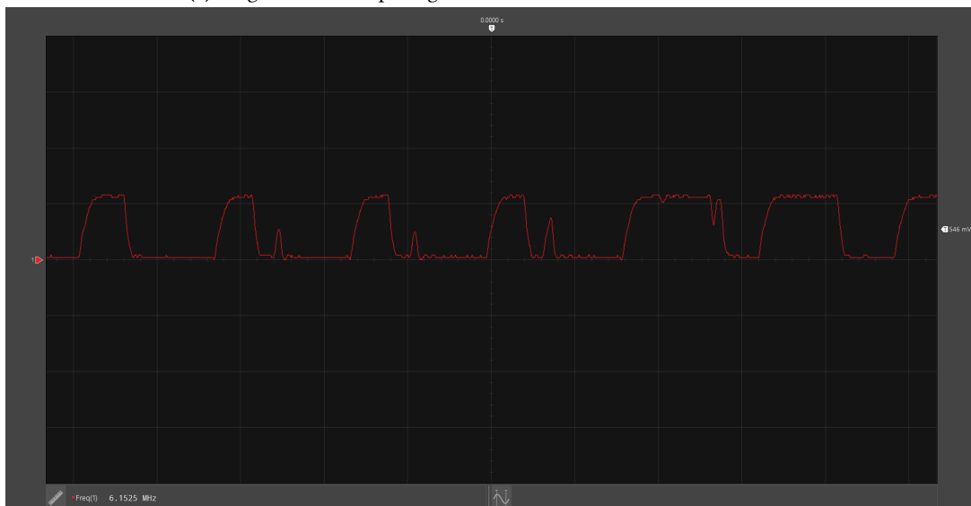
(b) Ring oscillator output signal of an irradiated GateMate FPGA
