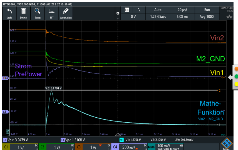
Abbildung 99: Regler R2 – Sourcemeter 1.5 A, externe Referenz 0.6 V, V_{wave} = 5 V , PrePower
