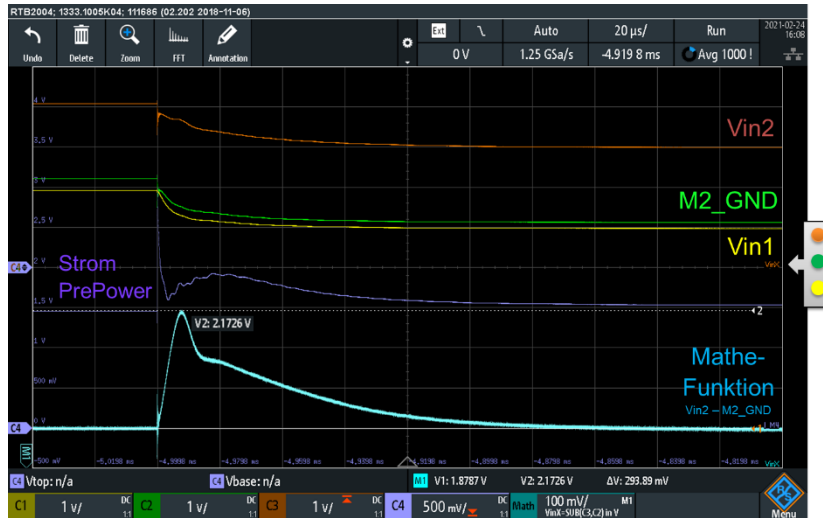
Abbildung 98: Regler R2 – Sourcemeter 1.5 A, interne Referenz, V_{wave} = 5 V , PrePower
