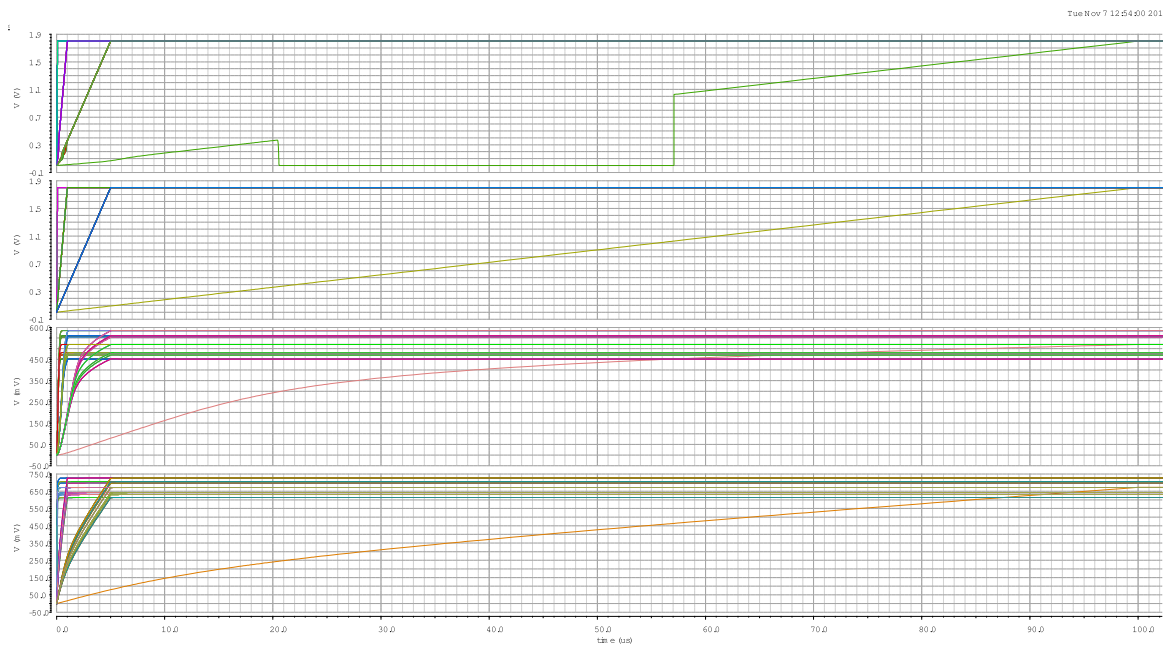
Figure 3.26: POR fast transient simulation using two MOSFETs in series with comparator filter
