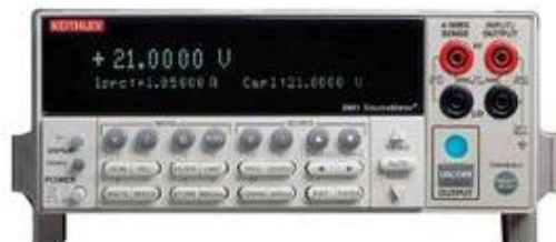
Abbildung 3.8: Sourcemeter Keithley 2401 [Keib]
