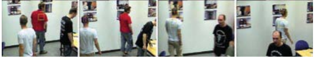
Figure 7. Interactive selection of another target object. Frames of sequence TS3. In the second image the man with the white T-shirt is selected for tracking instead of the previously tracked man with the red T-shirt. He is successfully taken over by the tracking module.
